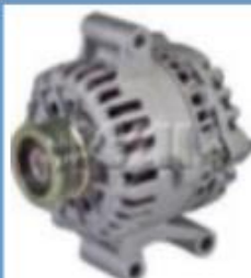
1-2350-11FD ALTERNADOR FORD 6G 110A FOCUS 2 TUBOS
